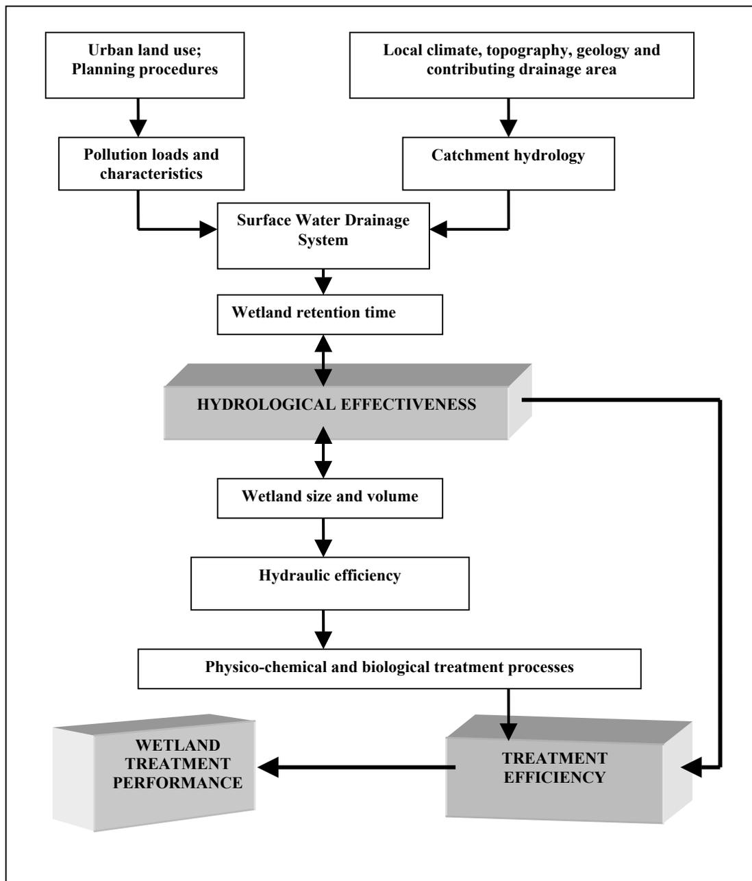
**Figure 3.1 Linkages and Interactions between Wetland Design Elements**
