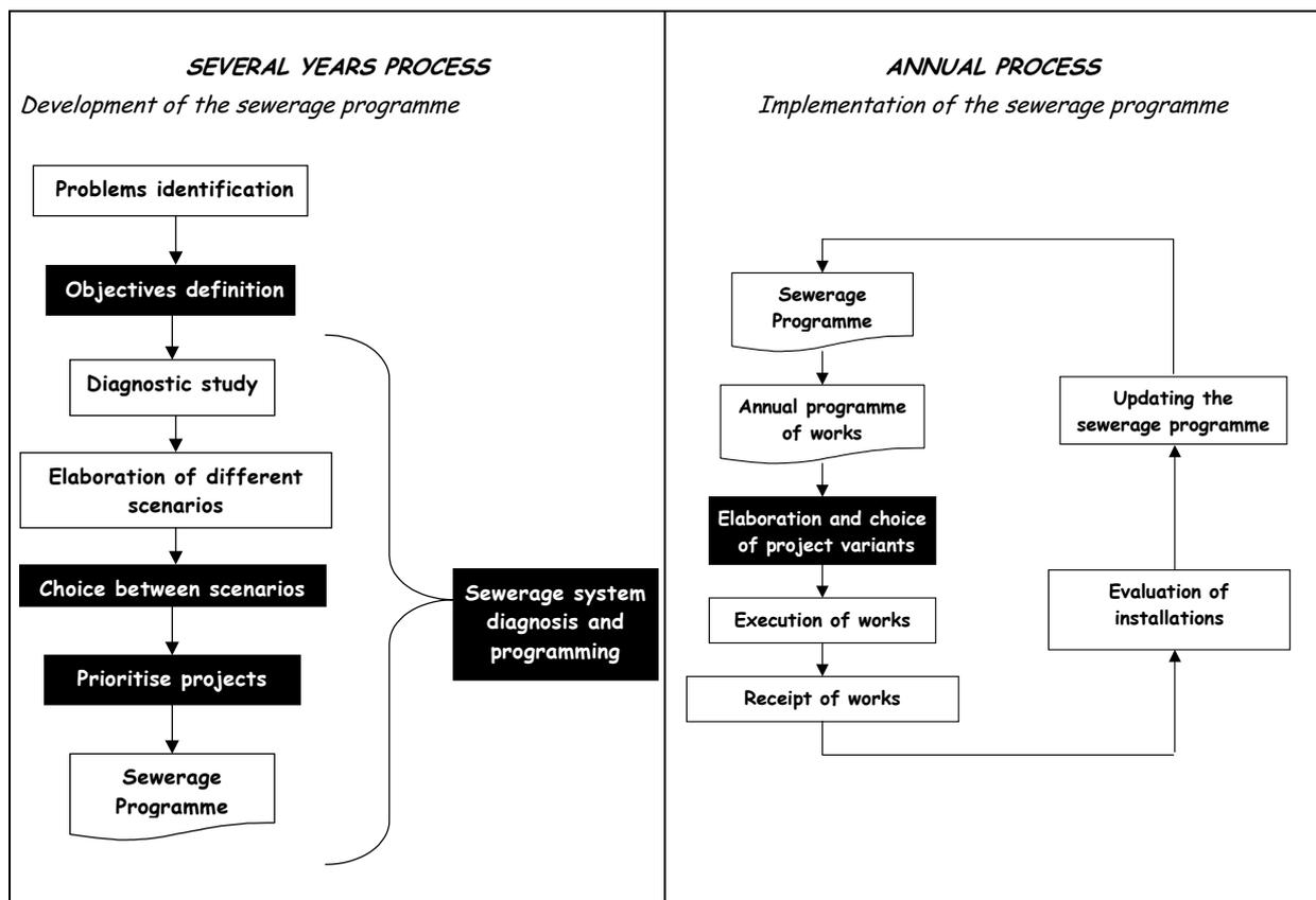
**Figure 8.1 Simplified Diagram of the Decision-Making Process for Urban Drainage in France**
