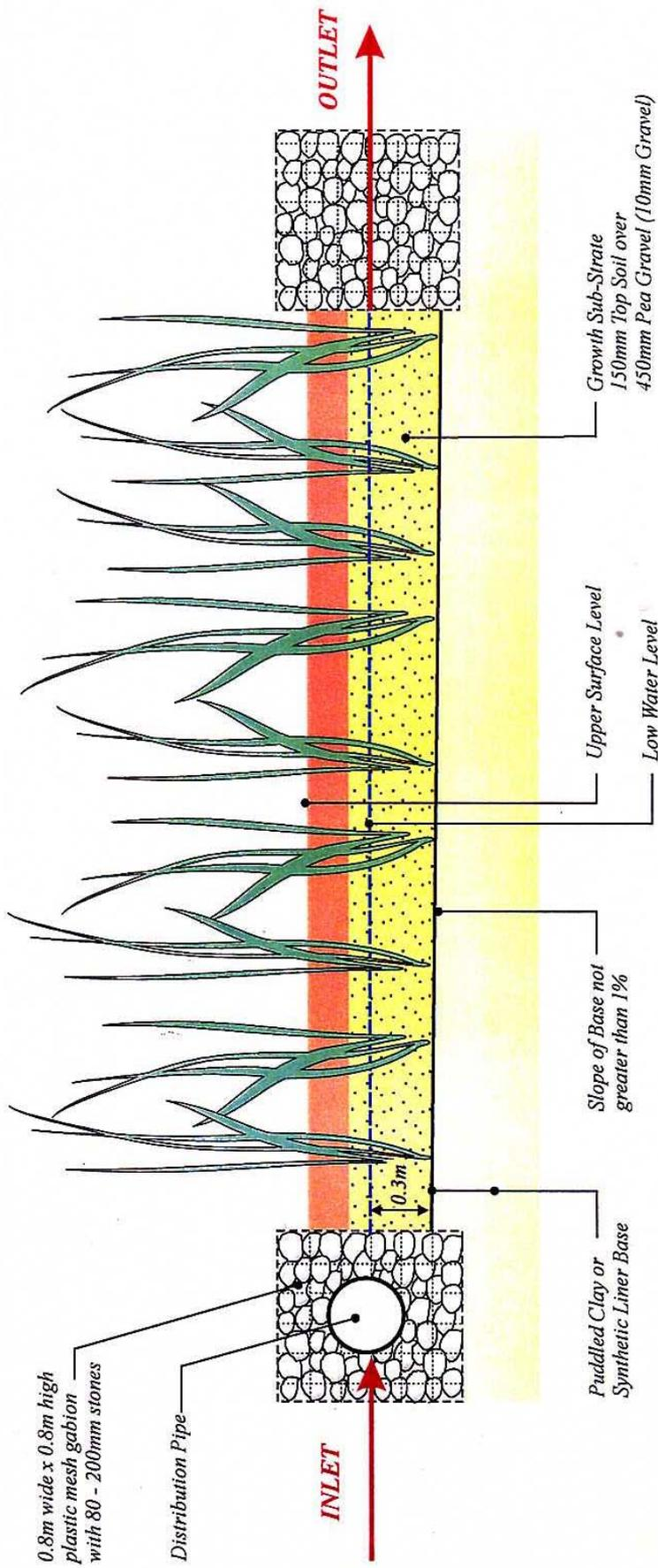
Figure 3.3 Section Through SubSurface Constructed Wetland
