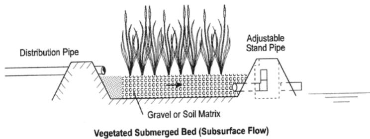
**Figure 1.2b. A SSF Constructed Wetland Illustrative Cross-section**
