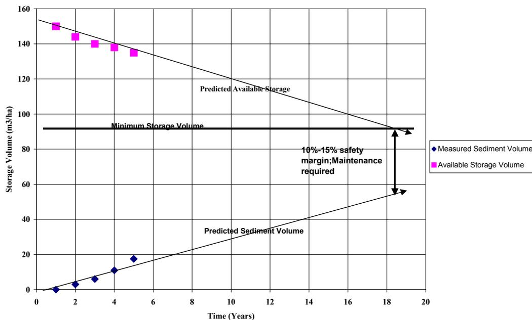
**Figure 4.4 Predicting Sediment Removal Maintenance Requirement Time**
