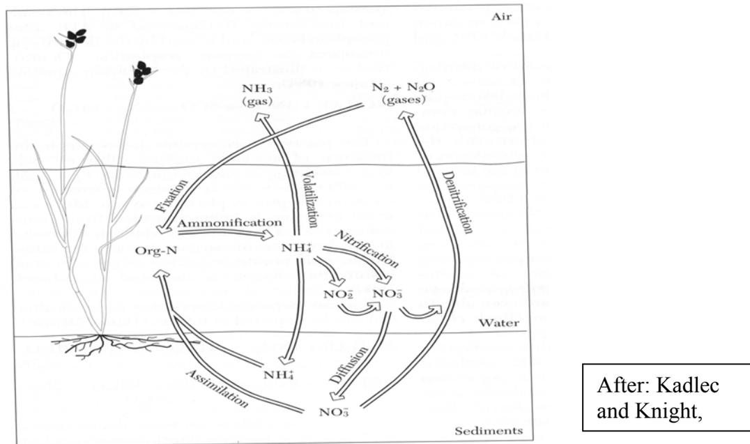
**Figure 1.3. Nitrogen Transformation in a Wetland System**
