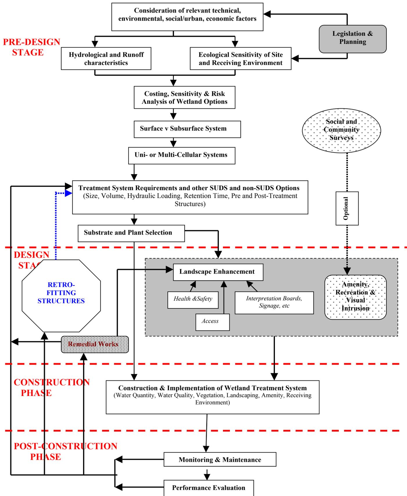
Figure 7.4 Process Diagram for the Design of Constructed Wetlands
