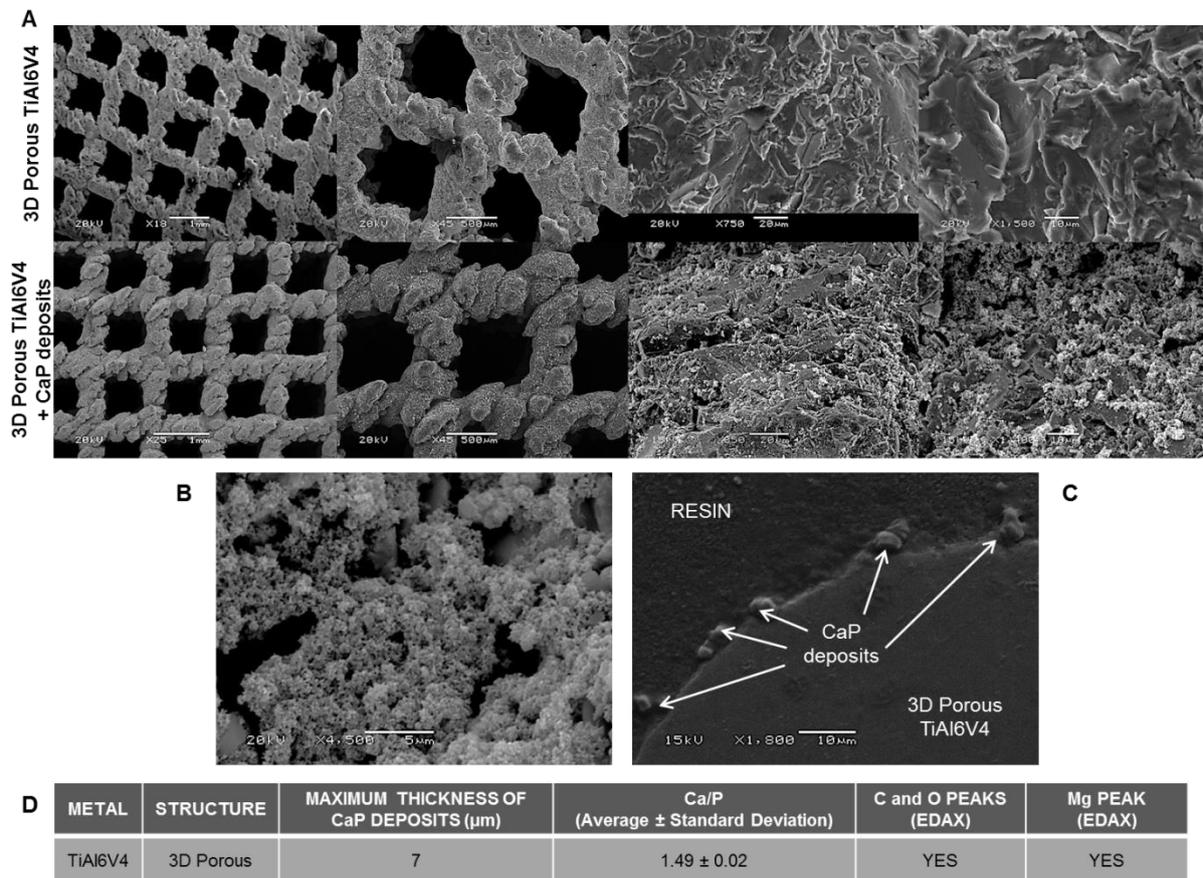
**Figure 9.** A) SEM comparison of 3D porous TiAl6V4 with and without CaP deposits. B) Representative SEM image of the amorphous nano-sized CaP particles deposited throughout the 3D porous TiAl6V4 structures. C) Cross-section of 3D porous TiAl6V4 showing CaP deposits inside the structure (SEM). D) Maximum thickness of CaP deposits as measured by SEM and summary of EDAX results.
