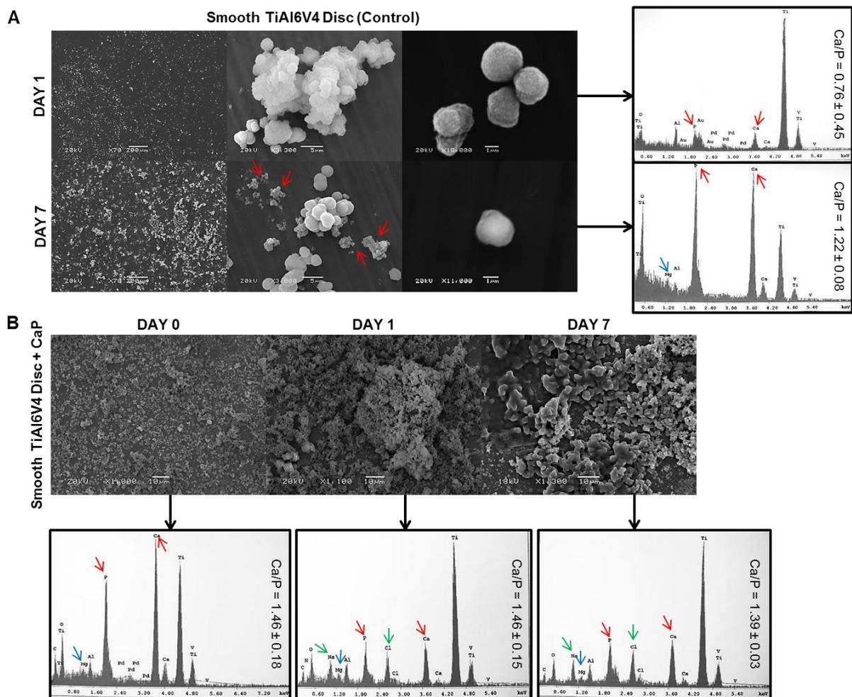
**Figure 6.** Apatite layer formation results. A) Smooth TiAl6V4 discs without CaP deposits (Control) and B) smooth TiAl6V4 discs with CaP deposits. Red arrows in SEM images point at mineral deposits of nano-sized particles. Red arrows in EDAX spectra point at Ca (main peak) and P peaks, blue arrows point at Mg peaks while green arrows point at Na and Cl peaks.
