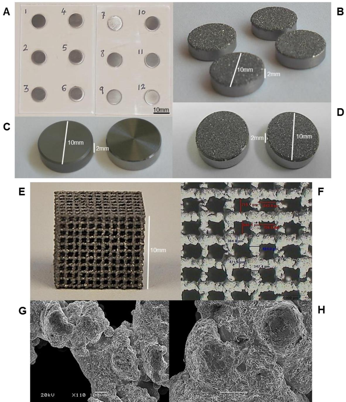
**Figure 1.** Materials used in this study. A) Ta discs after being polished showing a smooth surface; B) sand-blasted Ta discs showing a rough surface; C) TiAl6V4 discs before being polished to obtain a smooth surface; D) sand-blasted TiAl6V4 discs showing a rough surface. Polished or rough Ta and TiAl6V4 discs had identical macroscopic appearance. E) Macroscopic image of porous TiAl6V4 cubes; F) microscopic view of the porous
