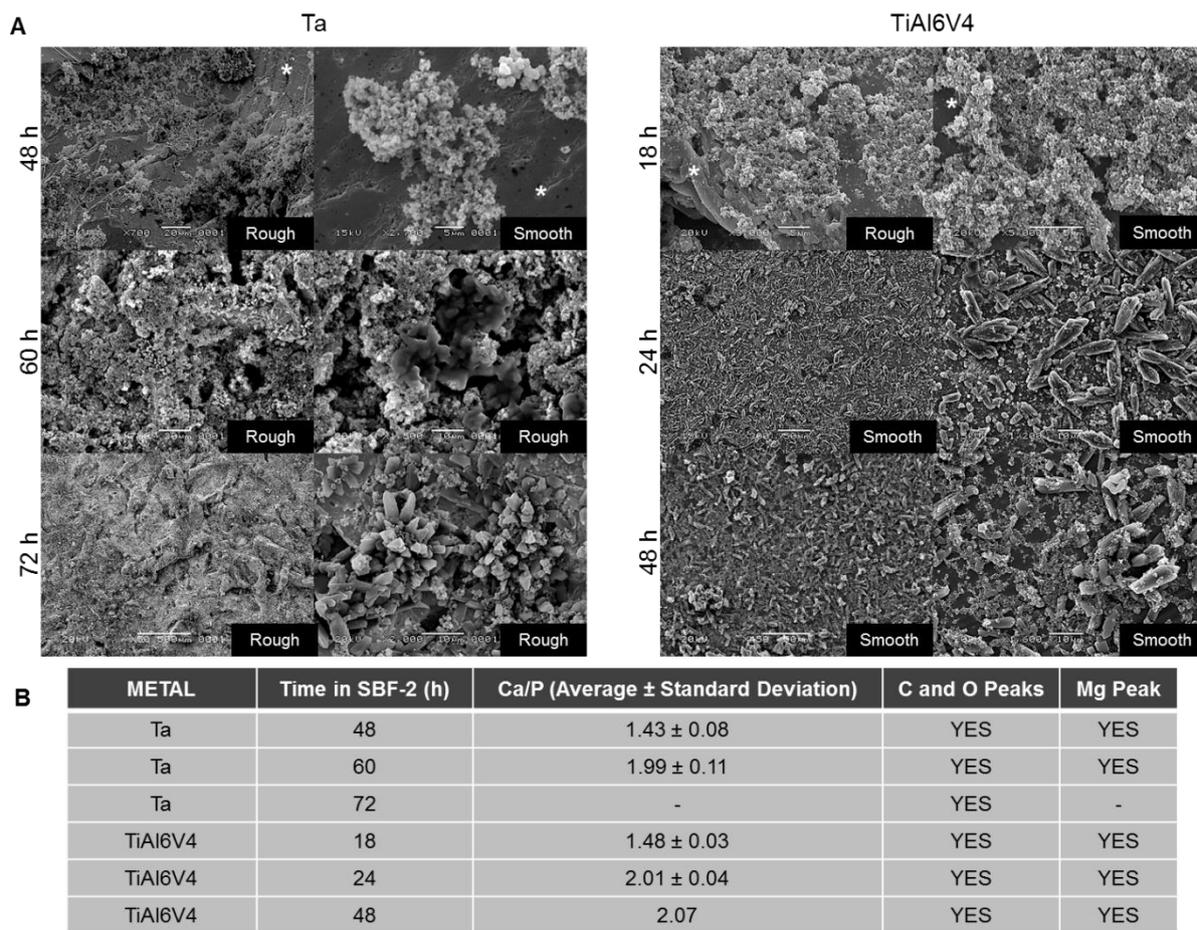
**Figure 3.** A) Representative SEM images for both Ta and TiAl6V4 showing the different mineral morphologies obtained with different immersion time in SBF-2. \*shows uncoated metal disc surface. B) Summary of EDAX results.
