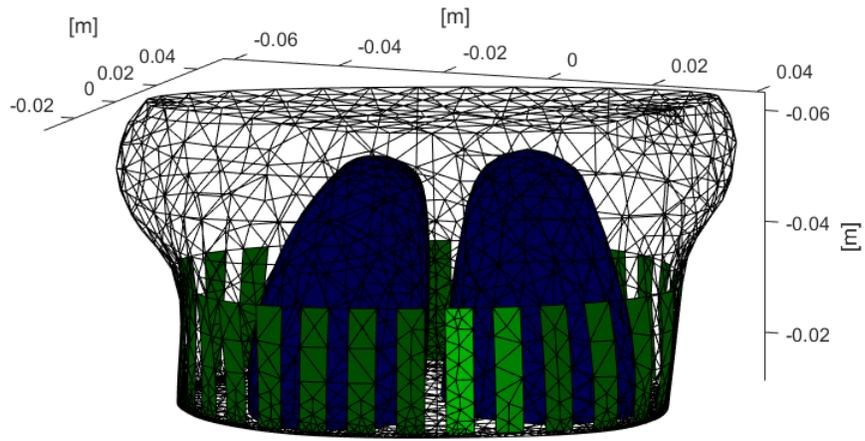
Figure 6: Neonatal phantom of torso meshed in Comsol and imported in the EIDORS toolbox.
