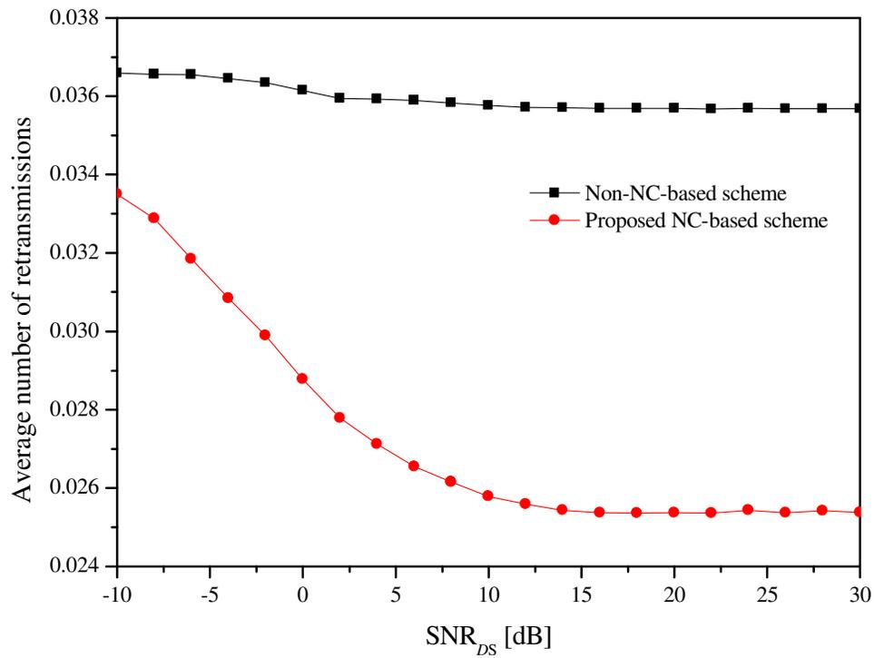
Fig. 6. Average number of data retransmissions per packet versus  $SNR_{DS}$  for Scenario 1.
