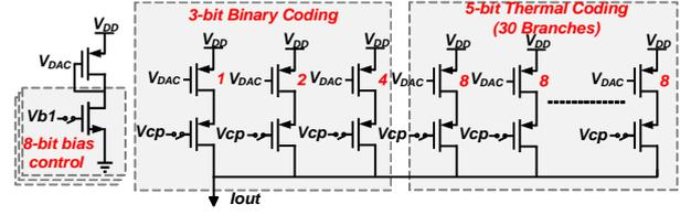
Fig. 4. Detailed schematic of the current DAC.
