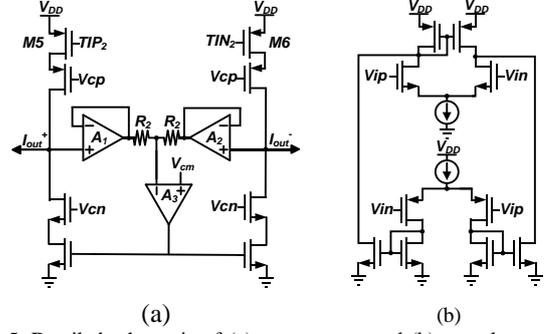
Fig. 5. Detailed schematic of (a) output stage and (b) complementary.
