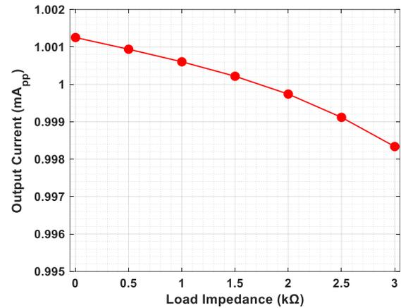
Fig. 10. The output current magnitude at 500 kHz with different load impedance values.
