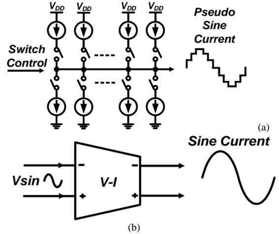
Fig. 1. Simplified diagram of (a) current DAC based CG and (b) V-I based CG.
