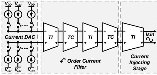
Fig. 2. Top-level block diagram of the proposed CG.
