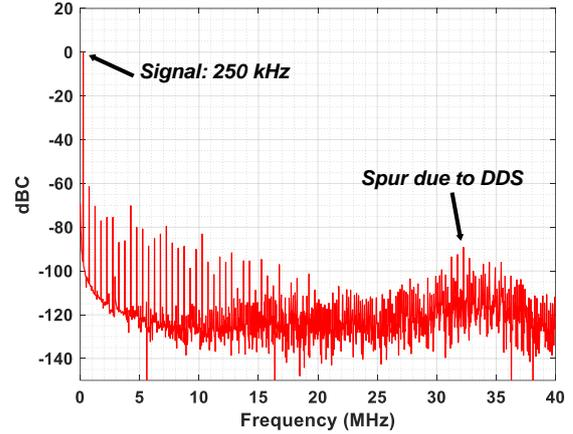
Fig. 8. FFT of the CG output current at a current magnitude of 1 mA<sub>pp</sub> and frequency of 250 kHz with a 1 kΩ load resistor.
