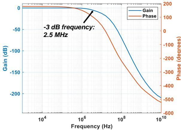
Fig. 7. ac response of the proposed fourth-order current-mode filter.
