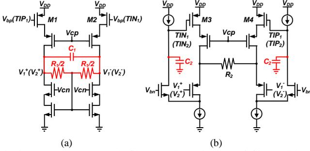
Fig. 3. Proposed current-mode filter. (a) TI based active RC filter and (b) TC based active GmC filter.
