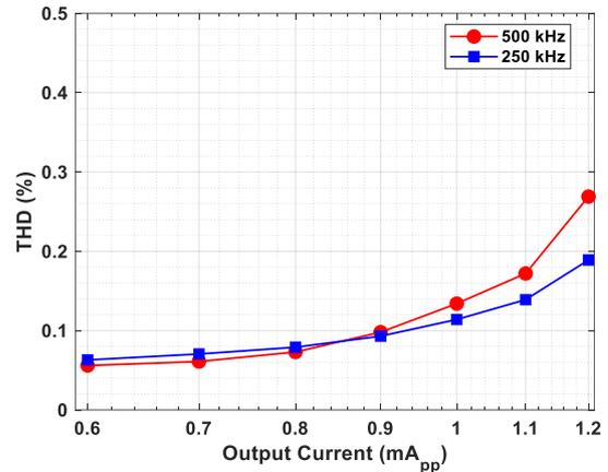
Fig. 9. THD versus different output current magnitude at signal frequencies of 250 kHz and 500 kHz.
