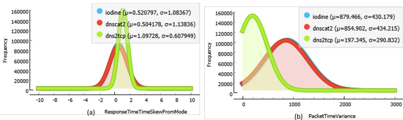
Fig. 9. Identifying the distinction between various malicious DNS tunnel tools, such as dns2tcp, DNSCat2, and Iodine for (a) ResponseTimeTimeSkewFromMode and (b) PcketTimeVariance feature.
