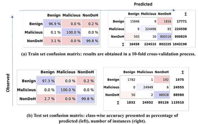
Fig. 4. Class-wise model performance for train and test set is shown in confusion matrices (a) and (b) respectively. For each case, class-wise accuracy is shown as a percentage of predicted on the left and a count of instances was shown on the right.
