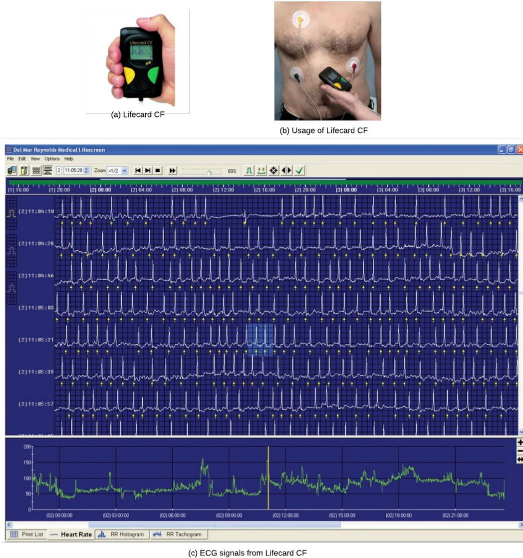
Figure 2.2: Lifecard CF gadget, usage and graphical representation of the ECG signals
